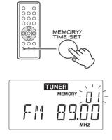
Within 5 seconds, select a preset channel to store the station using the PRESET buttons of the remote control unit.
